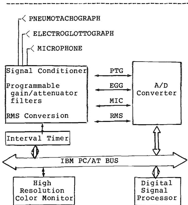
Figure 1. System configuration. Line connections indicate analog signals. Bar connections indicate digital I/O.
